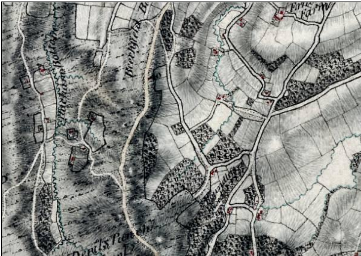
Figure 4. Example of an Ordnance Survey Drawing for Hindhead Common (produced in the field at 2 inches to 1 mile in 1810). This employs a more generalized set of symbols to indicate trees but the sophistication of the surveying is clear with careful attention to the depiction of relief through cross hatching and the inclusion of small wooded enclosures
