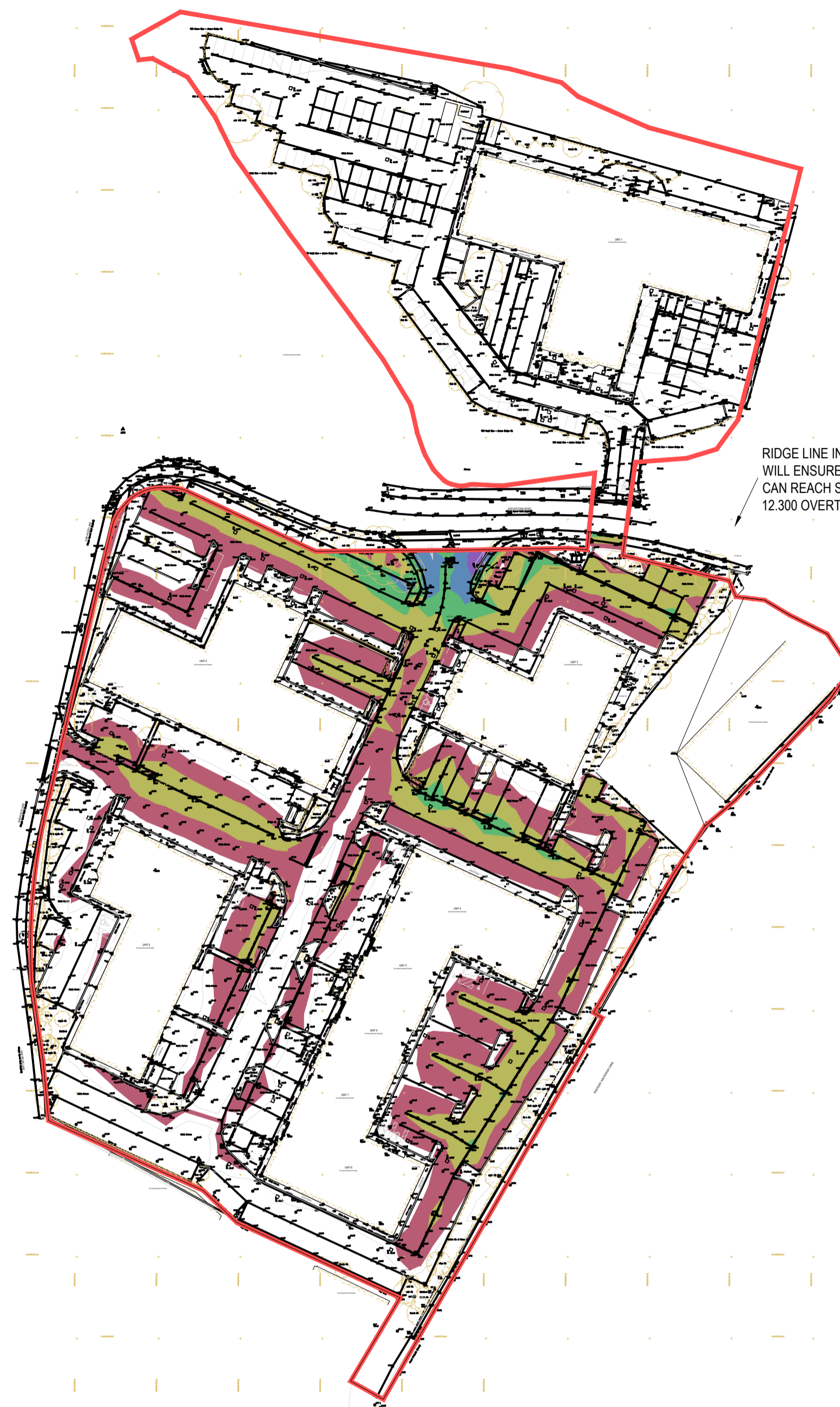
FLOOD VOLUME AT 12.460m AOD LEVEL = 750m 3 SCALE 1:1000
