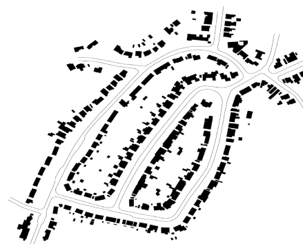
Figure: The Crescent, Egham showing how consistent building frontages can create irregular shaped perimeter blocks.
