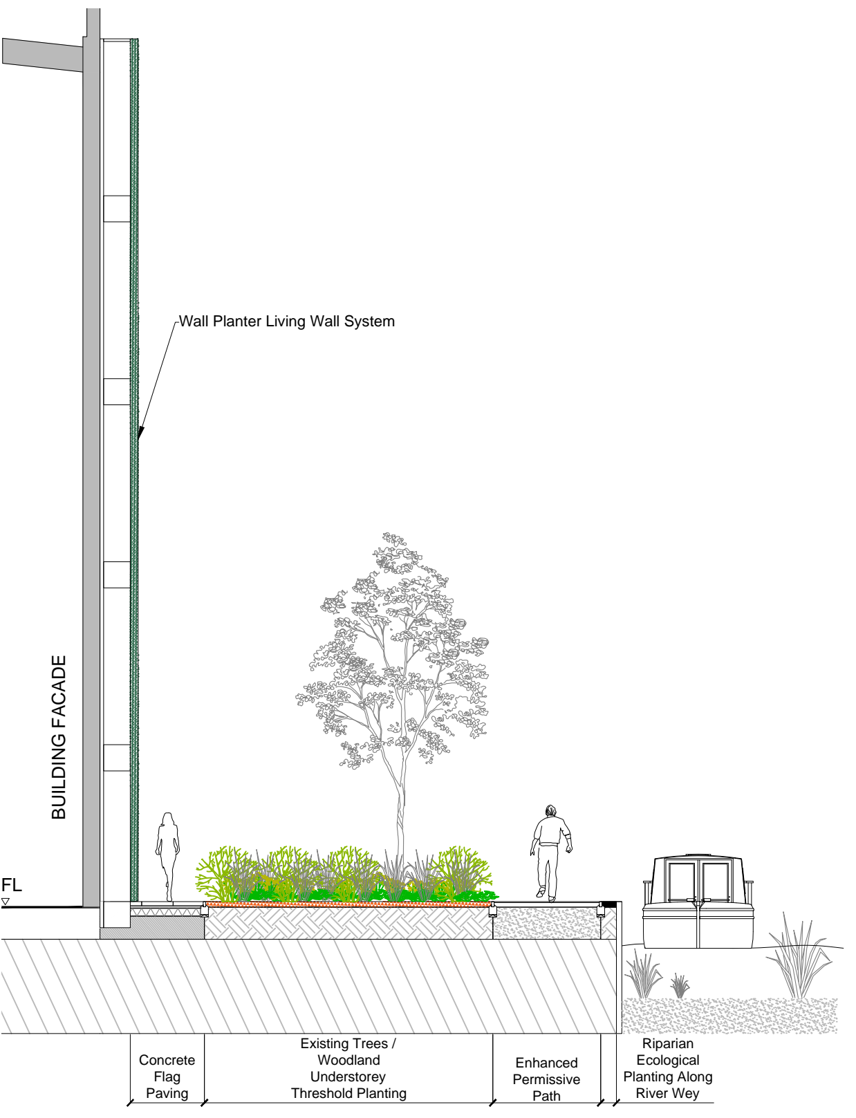
Section C-C Wall Planter and Riparian River Corridor Scale 1:100
