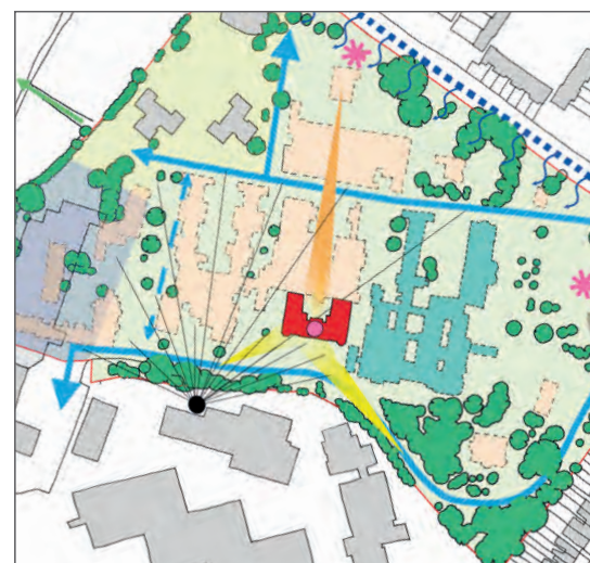
A site analysis diagram may typically show key routes, nodes, opportunities and different land uses, listed and existing buildings, trees, views and urban design features such as gateways and focal points.
