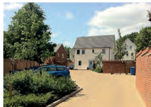
Rear court parking can be an acceptable solution if there is direct frontage to provide natural surveillance, and if high quality materials and landscape are used to create a pleasant environment.
