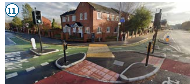
Case study: 'Cycle Optimised Protected Signals' (CYCLOPS) junction at Royce Road, in Hulme, south Manchester. Source: Google street view
