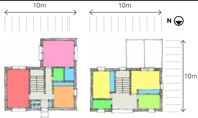
C2. L-shaped 3 bedroom house Either as a corner building or as an one-storey extension of the type B2
