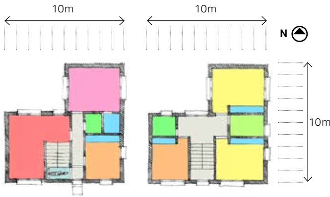
C3. L-shaped 4 bedroom house Either as a corner building or as a two-storey extension of the type B1
