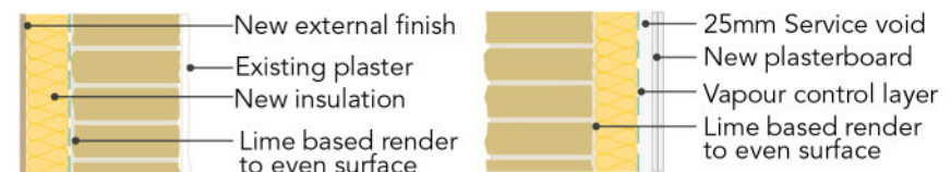
Externally insulated Stone Wall
