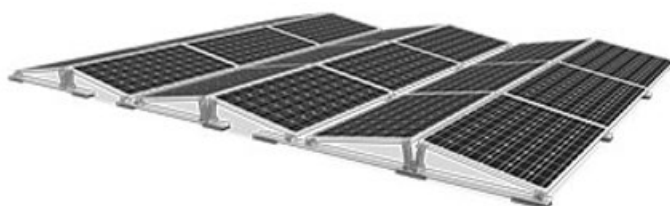
East/West facing concertina type solar arrays are usually the best solution for the flat roofs of blocks of flats. They generate less energy per panel than rows of south facing panels, but achieve much higher panel densities as they do not require large gaps between the rows to avoid interrow shading. (Source: K2 Systems)
