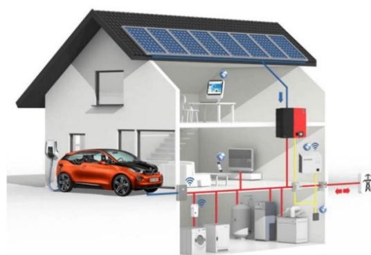
Smart controls and demand response measures in the home (Source: SMA Solar UK)
