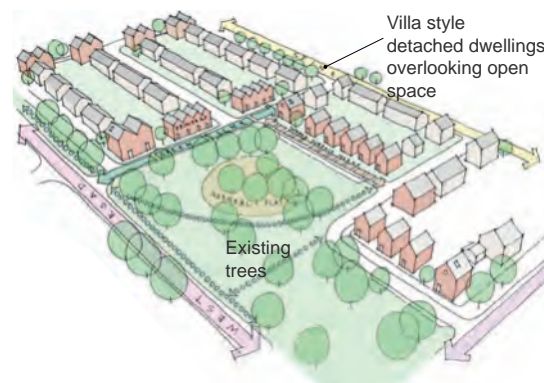
This layout demonstrates an approach to grouping different building types to define open spaces and streets - this creates consistency through rhythm of the built form and frontages, the materials, gardens and planting.
